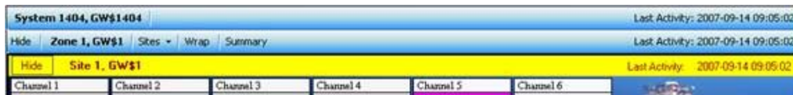
Figure 2.10 – A yellow site, indicating it is idle
